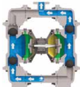
CONTAINMENT DUTY BALL WITH DIAPHRAGM DAMAGE DETECTION
