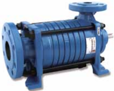
TCD – CONSTRUCTION FOR HEAT-EXCHANGE OILS UP TO 320 °C WITH A SIMPLE MECHANICAL SEAL WITHOUT COOLING, DERIVED FROM THE DIN 24258 STANDARD OF CHEMICAL PUMPS; BEARINGS ARE LUBRICATED WITH A BEARING OIL AND NOT WITH THE PUMPED FLUID AS IN COMPETITIVE PRODUCTS.
