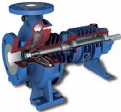
TBA – SELF-PRIMING HIGH-PRESSURE PUMP CONSTRUCTION WITH VERY LOW NPSHR, ABLE TO PUMP FLUIDS AT THEIR BOILING POINTS WITH MINIMUM CAVITATION RISK; COMPACT BEARING SHIELD, SHORT SHAFT AND COMPACT DIMENSIONS EXCLUDE VIBRATIONS, THUS EXTENDING THE LIFE OF THE BEARINGS AND SEALS.
